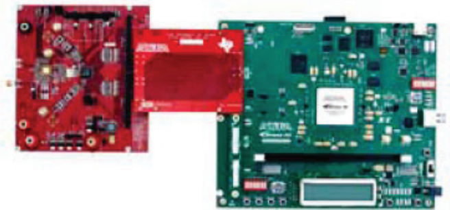
TI ADC Evaluation Module with Interposer Card Connection to Altera Development Kit
