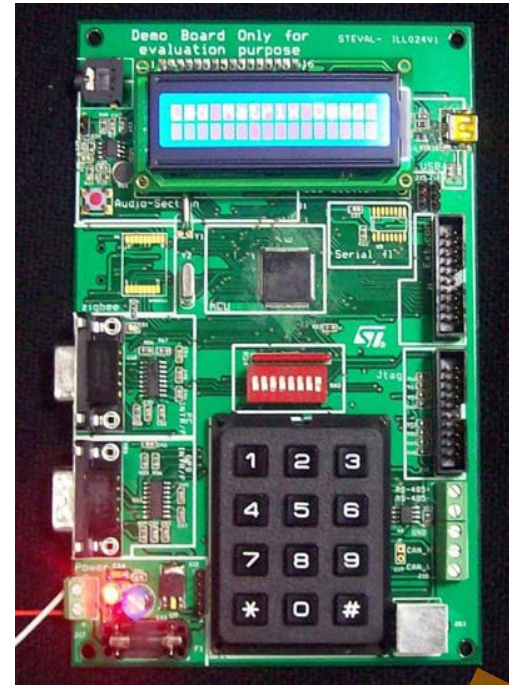
STEVAL-ILL024V1 LED Matrix Control Unit based upon STM32F103VB
