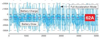
Peak levels should not be the determining factor when selecting relays. More importantly AVERAGE (RMS) current levels should be considered.
