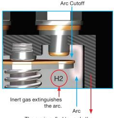
The arc is pulled towards the wall by permanent magnet.
