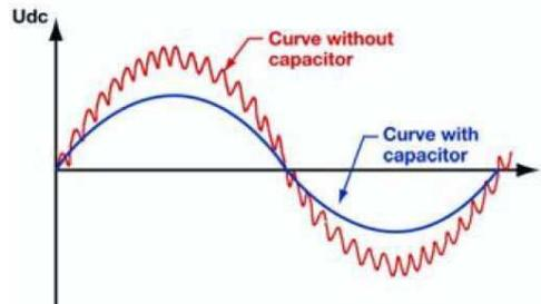
When in use, the ER series effectively stabilizes a device's voltage output. This capacitor will remove, or filter, any excessive spikes in voltage. By constantly absorbing and storing abnormal electrical outputs, the ER series will buffer uncharacteristic voltage values, creating a smoother output.
