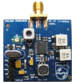
SA6x6DK OM13531 RF = 45 MHz; IF = 455 kHz
