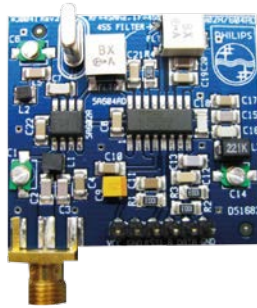
SA602AD + SA604AD OM13535 RF = 45 MHz; IF = 455 kHz
