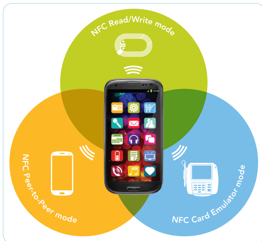
Figure 1. The three modes of NFC communication
