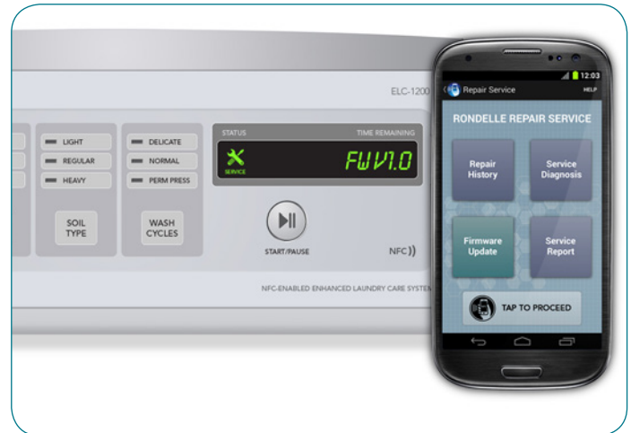
Figure 5. An NFC-enabled device facilitates appliance firmware updates and data delivery
