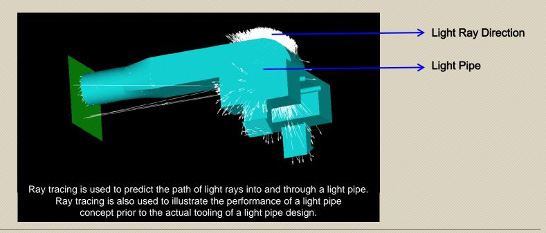
Ray tracing is a method of calculating the path of light through a light pipe through a virtual model Lumex uses state-of-the-art ray trace software with precise 3D CAD/CAM models for optimal light transmittance to ensure proper light pipe design. This advanced technology system helps to predict the direction of the light traveling through a light pipe, thereby eliminating costly and time-consuming steps and ultimately ensuring the most efficient design for a product.
