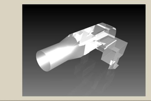
To ensure optimal light transmittance, ray tracing is completed in a three step process. First, a three dimensional model, representing an original design concept of a light pipe is created using 3D CAD software to scale. This model is an accumulation of the physical dynamic of a specific light pipe application (including any bends, angles and material for light transmission).
