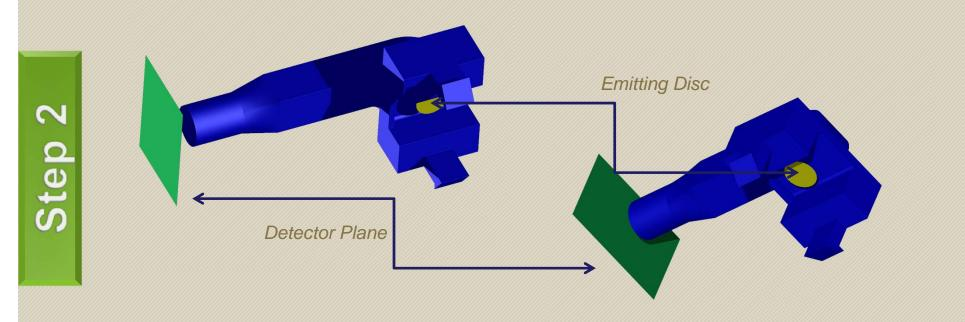
Next, an artificial LED is created, called an emitting disc, within the ray tracing program. The emitting disc simulates the intensity and the viewing angle of an LED, which is placed on the surface of a light pipe model. The detector plane is created in front of a surface where the light is intended to exit. The combination of these two planes in the ray trace program determines the amount of light transfer from LED to the emitting surface of a light pipe.
