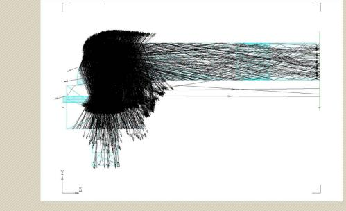
With a precise 3D model and proper LED viewing angle, it is then possible to run the design through Lumex's cutting-edge ray tracing technology to test the exact light output in terms of both uniformity and brightness. By measuring this light output via ray tracing, adjustments can be made to ensure that the most efficient light transmission path is identified and tested before any time or expenses are spent on tooling.
