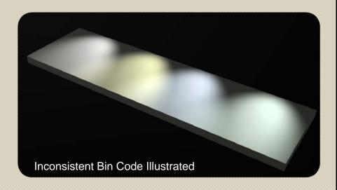
Multiple un-binned LEDs
