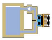
Since LA units require a pump to operate, many customers opt to incorporate a Re-Circulating Chiller into their system. This is a self contained unit that consists of an LA unit, pump, reservoir, power supply and temperature controller housed inside of a sheet metal casing. The temperature controller provides closed loop feedback control in order to maintain a specific outlet temperature of the liquid.
