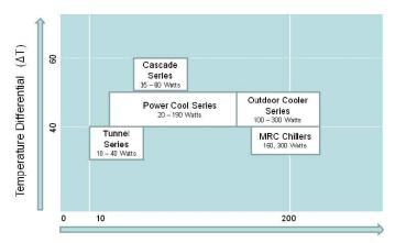
Heat Pumping Capacity (Watts)
