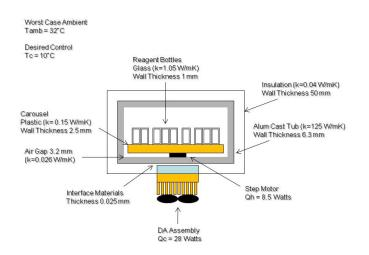
Running a simple 2D thermal analysis model can save time with selecting a TEA prior to actually purchasing it for trial and conducting validation testing. Consult with one of Laird Technologies' thermal design engineers for specific questions on how to run a thermal model, or have Laird Technologies run a thermal analysis of the application to confirm sizing of the TEA.
