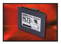
The EA KIT129-6 contains a 128 x 64 pixel LCD display with full graphics capability. An optional anti-glare, scratch-resistant touch panel with a 5 x 3 array of on-screen controls is also available. The control panel can be supplied with white text/graphics displayed against a blue background or black display on a white background. The blue/white version is the right choice for all indoor applications, whereas the black and white model is intended for outdoor use even in direct sunlight.
