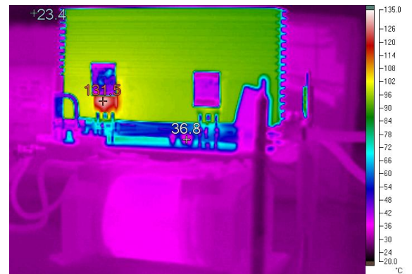
Fig. 14. Thermal performance at full load with IGW40N120H3 at 20KHZ
