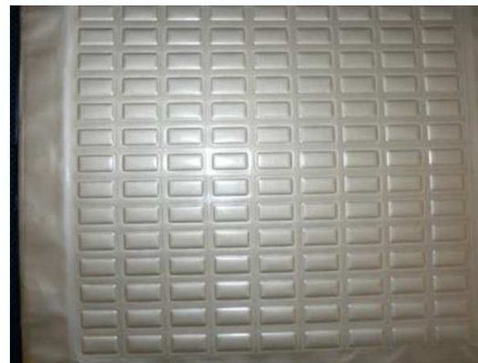
Wafer of 28x17 mm cells (144 cells)
