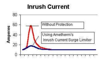
High inrush current can affect electrical systems by tripping fuses and circuit breakers unnecessarily. If inrush current protection is not in place, relays and fuses must be used that are rated higher than any possible inrush current. Inrush current can also cause pitted contacts on switches and relays due to the arcing of the contacts.
