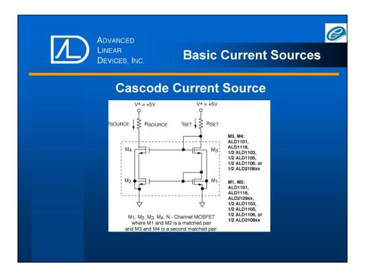
A full cascode current source can also be built with further expanded specs. The entire circuit can be operated in deep sub-threshold mode.
