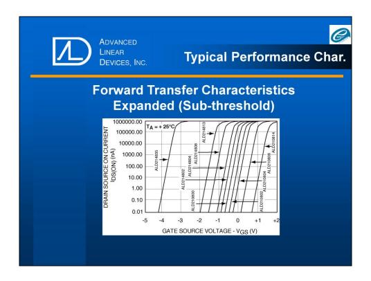
Looking closer at the IDS vs.VGS curve but with a log drain current vertical axis and linear horizontal gate source voltages, the vertical axis is now from 0.01nA or 10pA, to 1,000,000 nA which translates into 1.0mA which is a tiny part of the first curve. This current range spans over eight orders of magnitude.
