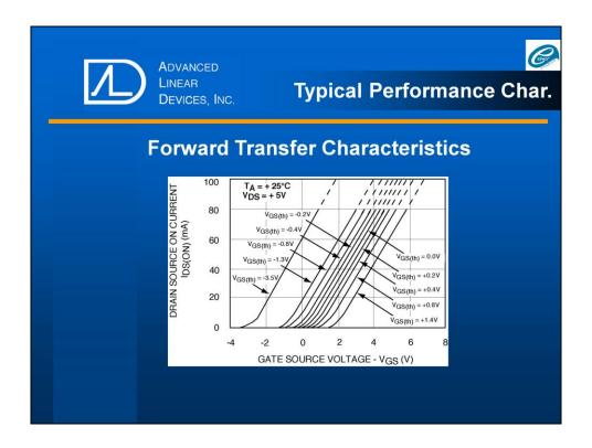
Here is a typical IDS (output) vs VGS (input) curve for this MOSFET product family. The vertical scale current range on this graph goes from 0 to 100 mA and gate voltage range goes from -4V to +8V (horizontal scale).
