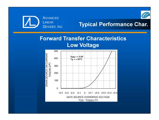
The same IDS vs. VGS curve at a low drain current range and low gate voltage range. Vertical scale is 0 to  $500\mu A$ , horizontal scale is -0.4V to +0.5V.
