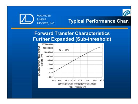
This graph describes exactly the same device and the same IDS current vs. VGS gate voltage relationship, except on a different horizontal unit scale. This gives yet another curve that looks different from the previous graphs.
