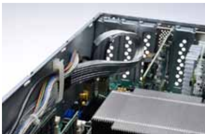
Flextronics server with 3M™ High Routability Internal miniSAS Twin Axial Cable Assembly inside
