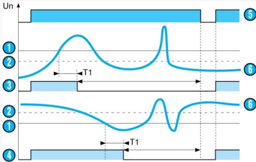
When the value of the controlled voltage, AC or DC, reaches the threshold  $U_e$  displayed on the front face, the output relay changes state at the end of a time delay  $T_1$ , which can be set on the front face at between 0.1 and 3s and remains latched in this position.
