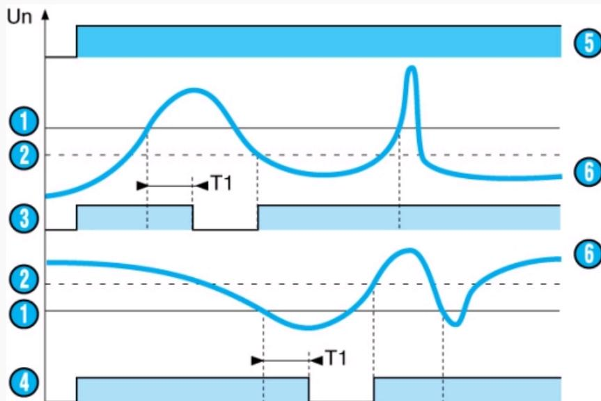
When the value of the controlled voltage, AC or DC, reaches the threshold  $U_e$  displayed on the front face, the output relay changes state at the end of a time delay  $T_1$ , which can be set on the front face at between 0.1 and 3s.
