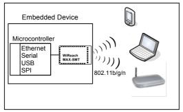
Nano WiReach MAX-SMT makes adding Internet connectivity to embedded devices a breeze. It does not require any kind of WiFi driver development on the host CPU, and its multiple interfaces (UART, SPI, RMII and USB 1.1) minimize the need to redesign the host device hardware.
