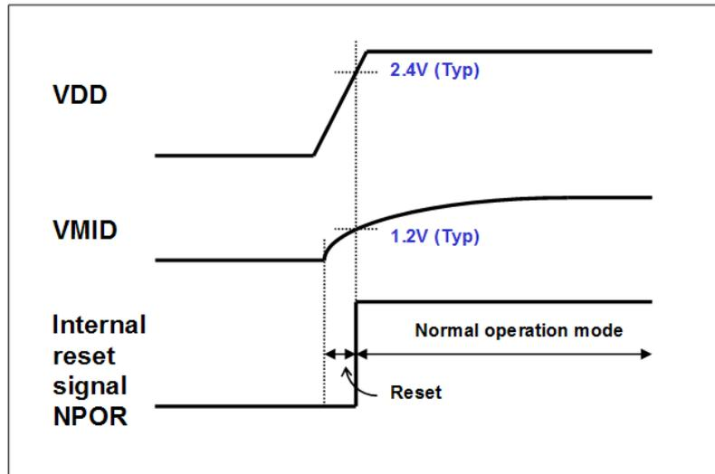
Figure 4 Generation of Internal NPOR at Power-On-Reset
