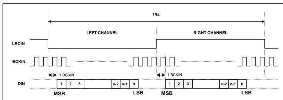
Figure 6 I<sup>2</sup>S Mode Timing Diagram
