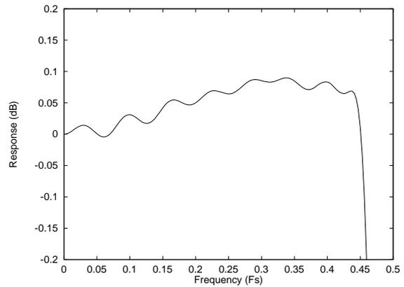
Figure 8 DAC Digital Filter Ripple -44.1, 48 and 96kHz
