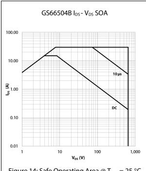
Figure 14: Safe Operating Area @ T<sub>case</sub> = 25 °C
