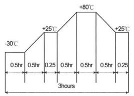
The diaphragm will be measured after being placed at +25°C for 4 hours. The value of the resonant frequency should be ±10%, the value of the electro static capacitance should be ±20% compared to the initial measurements. The resonant impedance should be 2,000  $\Omega$ max.
