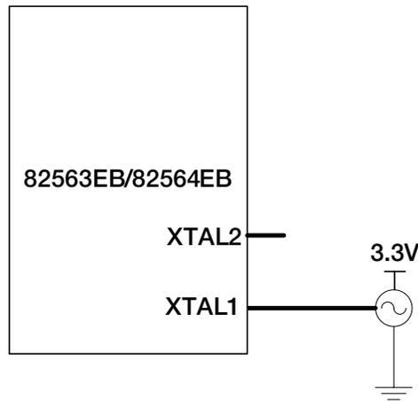
Figure 9. External Clock Oscillator Connectivity to 82563EB/82564EB
