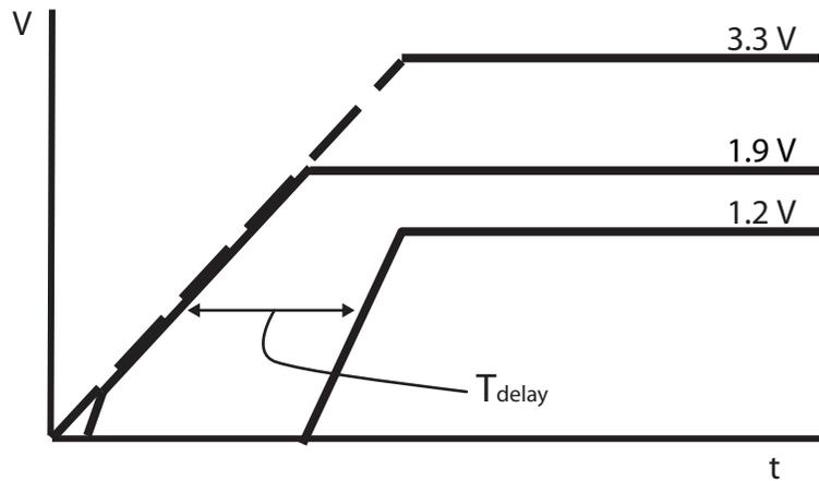
Figure 4. 82563EB/82564EB power up sequencing with internal regulators
