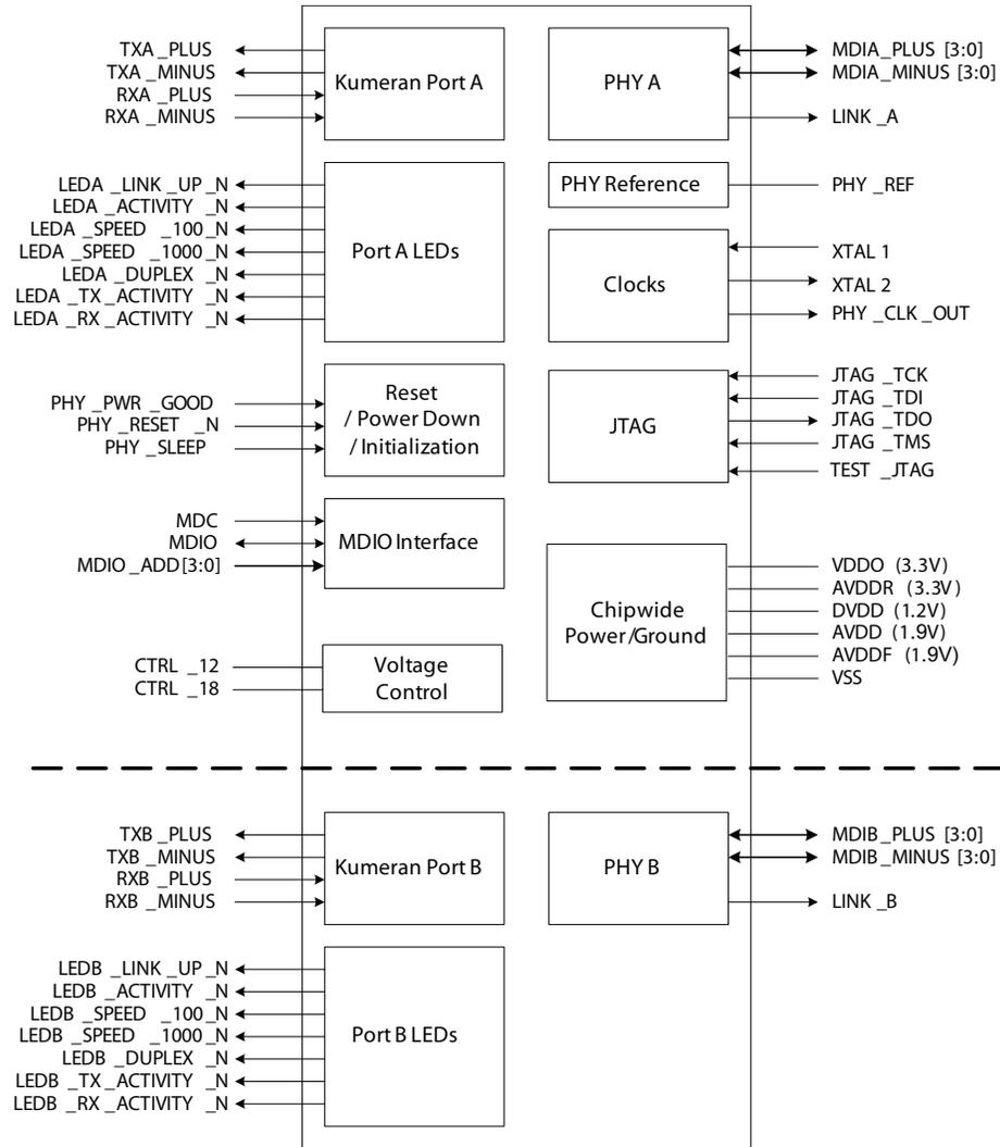
Figure 13. 82563EB/82564EB Interfaces
