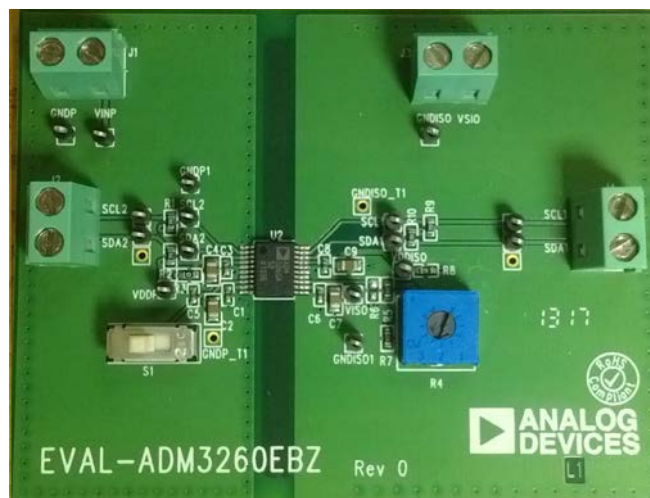
Figure 1. EVAL-ADM3260EBZ Evaluation Board
