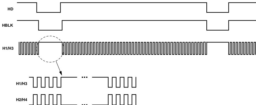
Figure 12. Horizontal Blanking Example Showing HBLKTOG1_0 = 0, HBLKMASKPOL = 0, and HBLKTOG2_0 = 3
