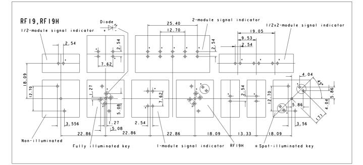
\*The LED may be positioned either on the left-hand or right-hand side. Standard version: LED on left-hand side View on component side, all hole diameters 1.1 +/- 0.1 mm
