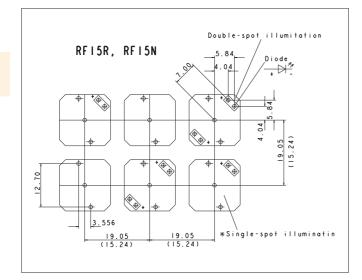
View on component side All hole diameters 1.1 <sup>+/- 0.1</sup> mm PCB layout keyswitch 1/400" grid
