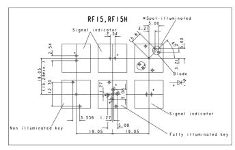
View on component side, all hole diameters 1,1  $^{\scriptscriptstyle +\!/-0,1}$  mm
