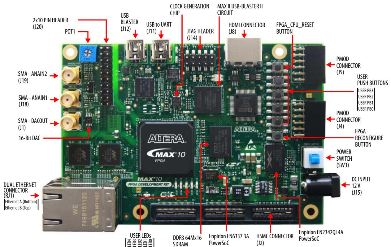
Figure 1-2: MAX 10 FPGA Board Components (Bottom)
