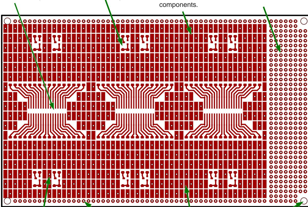
Every second SMT pad has an unplated hole for easy connection to the ground plane. Just insert a wire and solder.
