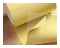
Sil-Pad 1100ST (Soft Tack) is a fiberglassreinforced thermal interface material featuring inherent tack on both sides. The material exhibits excellent thermal performance at low mounting pressures. The material is supplied on two liners for exceptionally easy handling prior to auto-placement in high-volume assemblies. The material is ideal for placement between an electronic power device and its heat sink.
