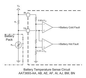
Figure 4: Battery Temperature Sensing Operation.
