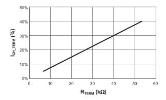
Figure 3: Charge Termination Current vs. R<sub>TERM</sub>.
