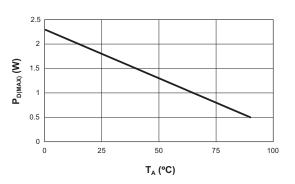
Figure 5: Maximum Power Dissipation Before Entering Thermal Loop.
