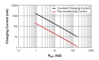
Figure 2: Charging Current vs. R<sub>SET</sub> Values.
