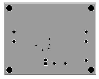
Figure 7: AAT3693 Evaluation Board Middle 1 Layer Layout.
