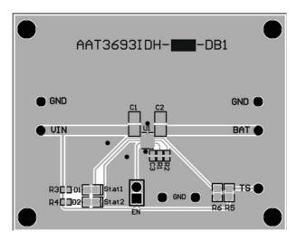
Figure 6: AAT3693 Evaluation Board Top Side Layout.
