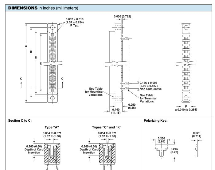
When ordering polarizing keys individually, specify by the Model Number: PK-7 between contacts. Hand insertion tool, TPK-7, provided upon request
