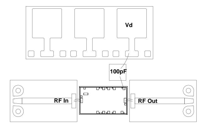
All DC connections may be brought in from either side of the chip (Use Pad 6 or 8) 0.01uF external Cap is recommended on Drain
