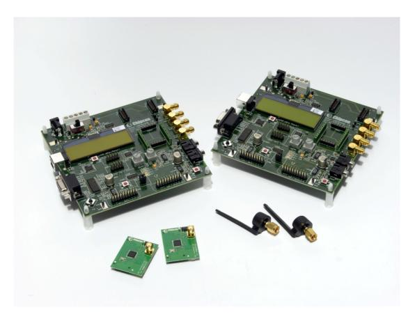
A SmartRF04EB and a CC2430EM platform can easily be set up to communicate with another platform of the same kind. These platforms can be used for testing and development of both hardware and software.
