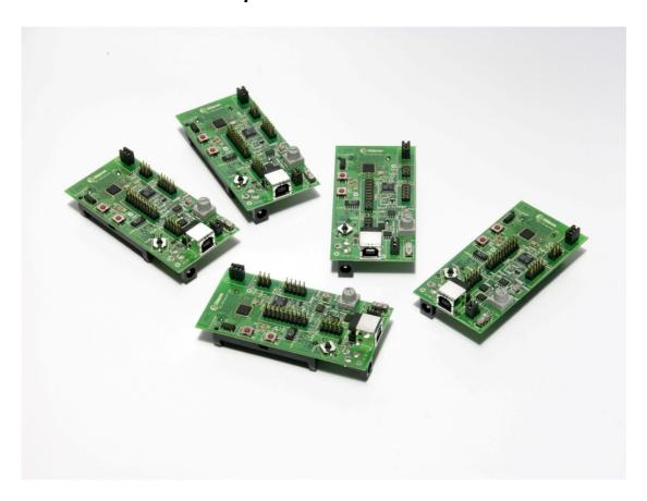
The CC2430DB can be used out-of-the-box to form self-configuring ZigBee™ networks. It is perfectly suited for ultra-low power and sensor applications. Because it includes a USB interface the CC2430DB can connect directly to a PC and to run the packet sniffer or the In Circuit Emulator. The USB interface
