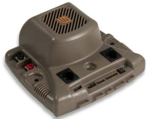
Figure 1. Brushed DC Motor Control Module
