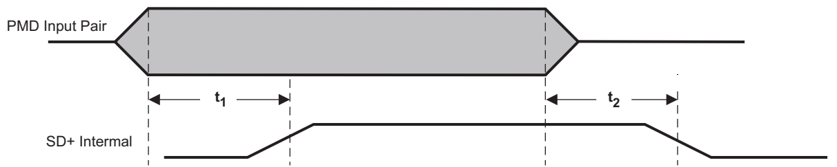
Figure 9-20. 100Base-TX Signal Detect Timing
