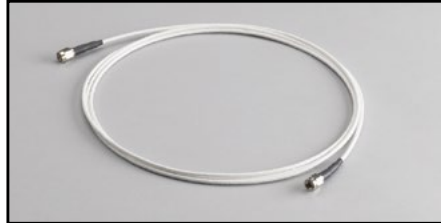
CA-404B: 2m (6.5 ft) RG188 coax cable terminated with an SMA male plug on each end, 50 \Omega impedance.
