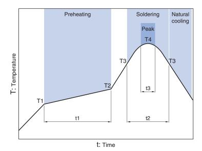
Preheating Soldering Peak Temp. Temp. Time Temp. Time Time T2 T3 T4 t3 150°C 180°C 250 to 260°C 60 to 120s 30 to 60s 230°C 10s max.
