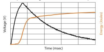
When using the test method indicated below, the amount of Energy dissipated by the varistor must not exceed the Load Dump Energy value specified in the product table.
