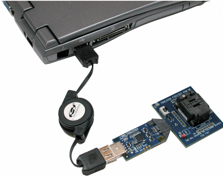
Figure 5. ToolStick Socket Platform Connected to PC
