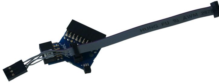
Figure 2-10. Atmel-ICE AVR Probe Connection
