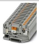
Test disconnect terminal block, Connection type: Push-in connection, Screw connection, Cross section: 0.5 mm² - 10 mm², AWG :20- 10, Width: 8.2 mm, Color: gray, Mounting: NS 35/7,5, NS 35/15
