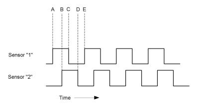
As shown above, this means that after sensor 1 goes high (A), sensor 2 then goes high (B) as the encoder continues to rotate. Then, as the encoder continues to spin, sensor 1 goes low (C), and then sensor 2 follows (D). Because sensor 1 went high before sensor 2 (A to B), it indicates that the encoder disk is rotating in one direction (in the case of a robot, either forward or reverse). If sensor 2 went high before sensor 1, then the disk is rotating in the opposite direction.
