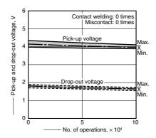
6-(2). Electrical life test (Lamp load)
