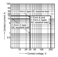
1-(2). Max. switching capacity (2 Form C)
