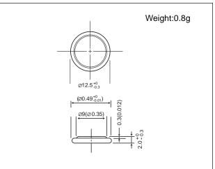
Note: This bare cell diagram is for size reference only. Please refer to the tab configurations at the end of this section for available tabs.
