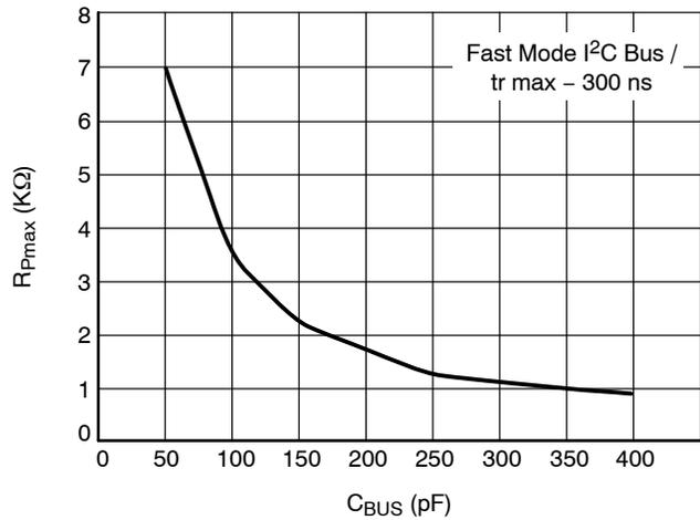
**Figure 5. Maximum  $R_P$  Value vs. Bus Capacitance**
