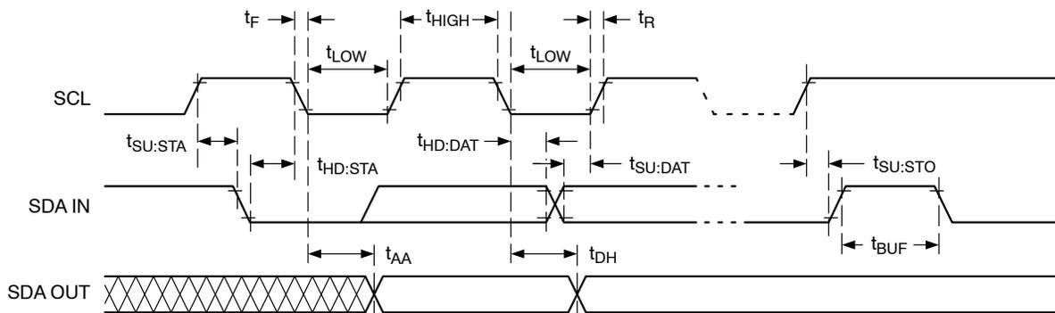
**Figure 3. I<sup>2</sup>C Serial Interface Timing**
