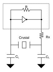
$$\begin{split} C_\text{L} &= 2^*(C_P - C_\text{S}),\\ \text{Where } C_P &= \text{Load capacitance of crystal}\\ C_\text{S} &= \text{Stray capacitance due to } C_\text{IN, } PCB, \text{ Trace etc.} \end{split}$$
