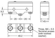
Note: With reverse action models (Z-15GM), the positions of NO and NC terminals are reversed.
