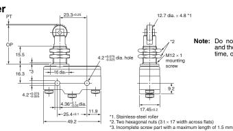
Note: Do not use the M12 mounting screw and the case mounting hole at the same time, or the case may be damaged.
