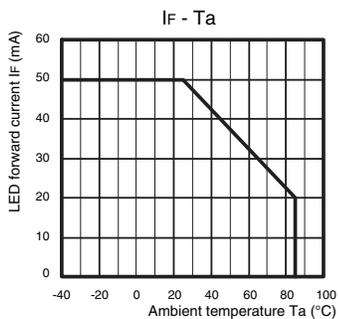
Continuous load current vs. Ambient temperature
