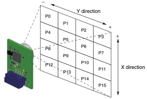
**Note:** Definition of view angle: Using the maximum Sensor output as a reference, the angular range where the Sensor output is 50% or higher when the angle of the Sensor is changed is defined as the view angle.
