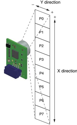
**Note:** Definition of view angle: Using the maximum Sensor output as a reference, the angular range where the Sensor output is 50% or higher when the angle of the Sensor is changed is defined as the view angle.
