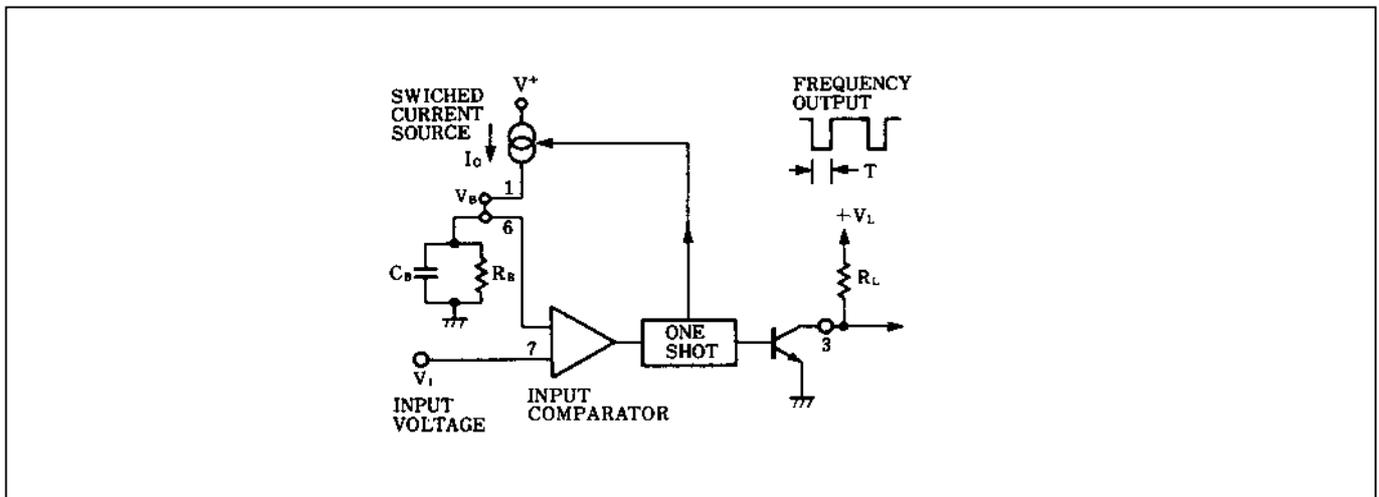
Figure 1. Simplified Block Diagram, Single Supply Mode
