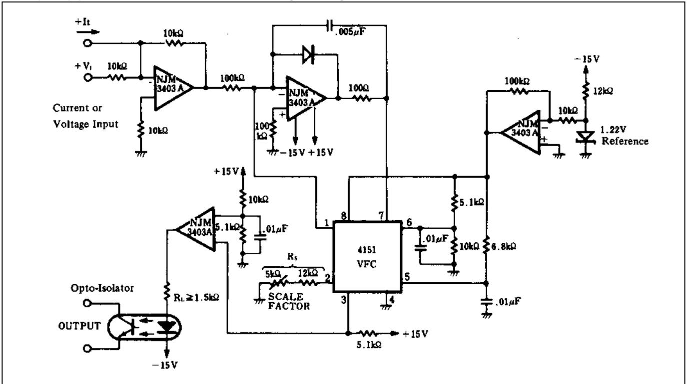
Figure 7. Opto-Isolated VFC
