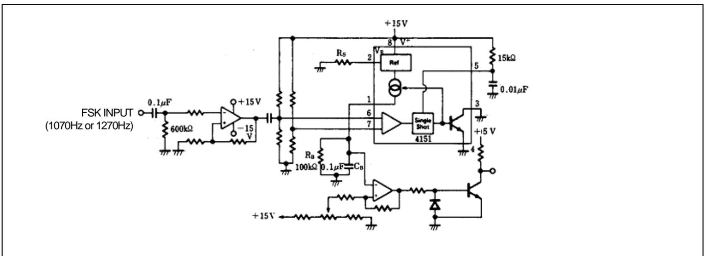
Figure 8. FSK demodulator
