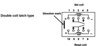
Double coil latch type (Reset position)
